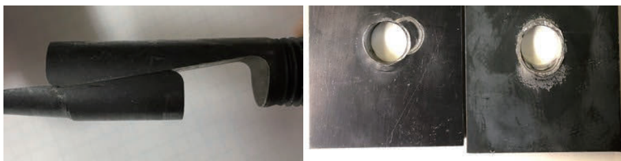
Fig. 13 Bolt & splice plate condition after experiment of 7 - plastic
