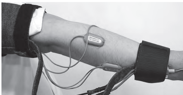
Fig. 5 Active Electrodes for EMG
